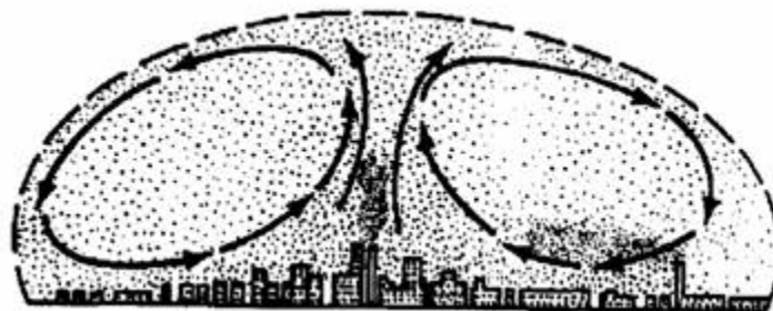
Figure 2: The heat generated within a large city tends to produce a circulatory air pattern which traps smog within a dome.
