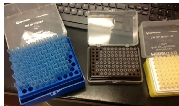
Micropipette tips for a P1000, a P10 and a P20 or P200
