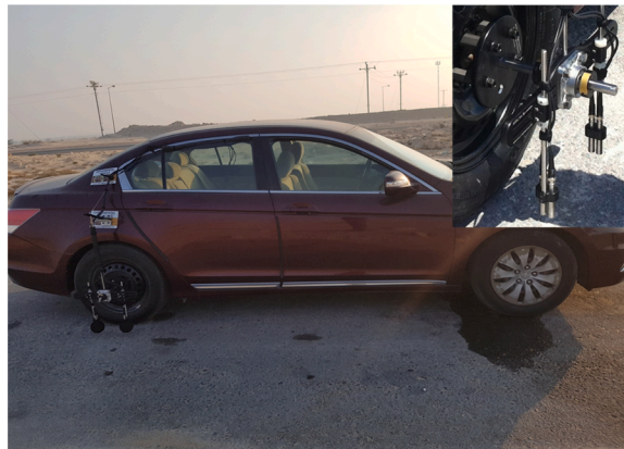
Fig. 3. OBSI noise testing setup.
