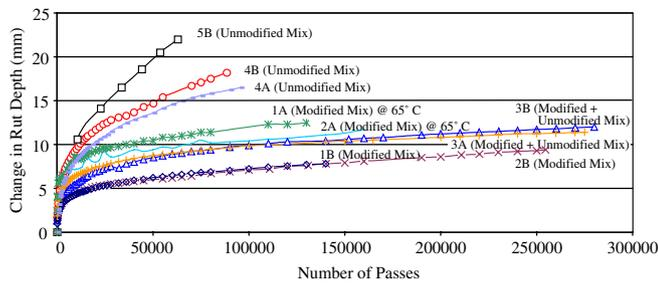
Fig. 5. Comparison of change in rut depth as measured by the differential surface profile method vs. number of passes in Phase II.
