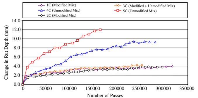
Fig. 4. Comparison of change in rut depth as measured by the surface profile method vs. number of passes in Phase I.
