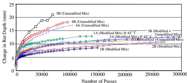
Fig. 6. Comparison of change in rut depth as measured by the surface profile method vs. number of passes in Phase II.
