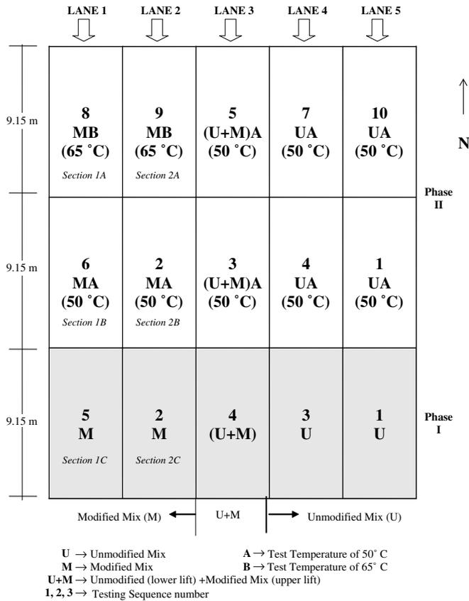
Fig. 3. HVS testing sequence (Plan view).
