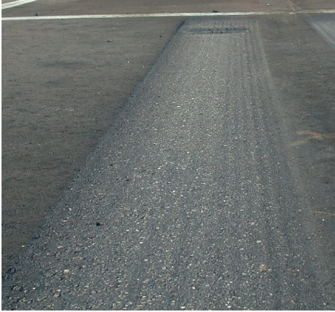
Fig. 16. Photo of Section 7A-W (uni-directional loading with 10 cm wander in 2.5 cm increments).
