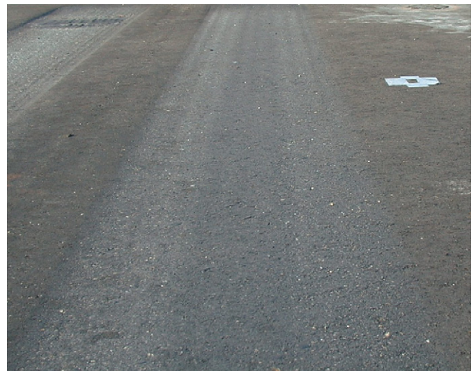
Fig. 11. Photo of Section 7A-E (bi-directional loading with 10 cm wander in 5 cm increments).
