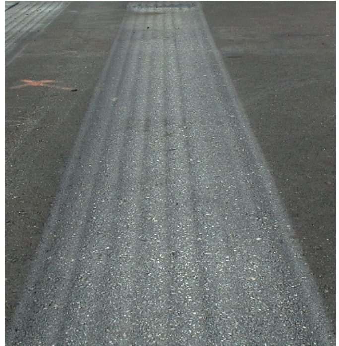
Fig. 10. Photo of Section 7B-E (uni-directional loading with 10 cm wander in 5 cm increments).
