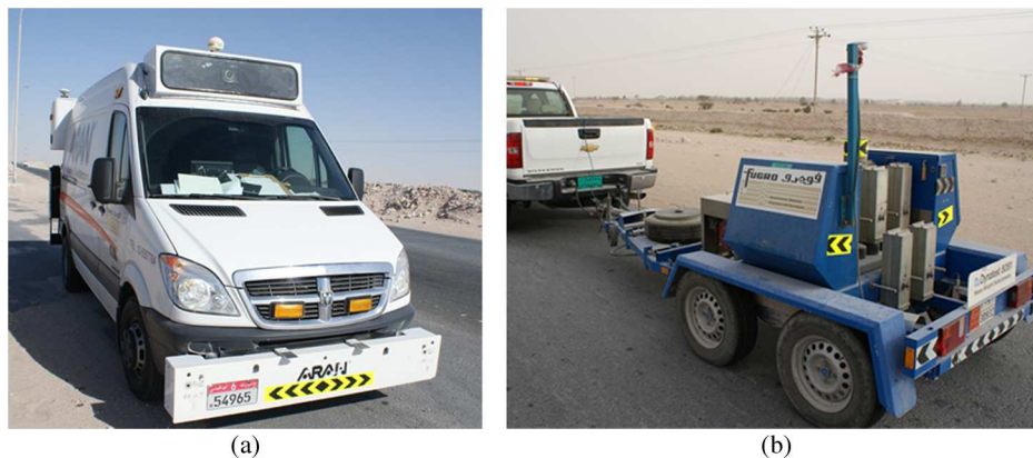
Fig. 4. (a) Automatic road analyzer vehicle collecting data from site; (b) FWD test conducted on the site
