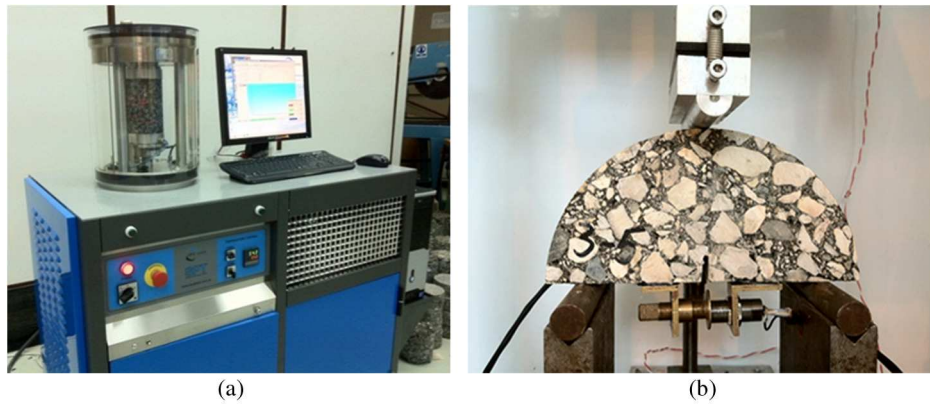
Fig. 6. (a) AMPT for dynamic modulus and flow number tests; (b) set up for monotonic SCB test
