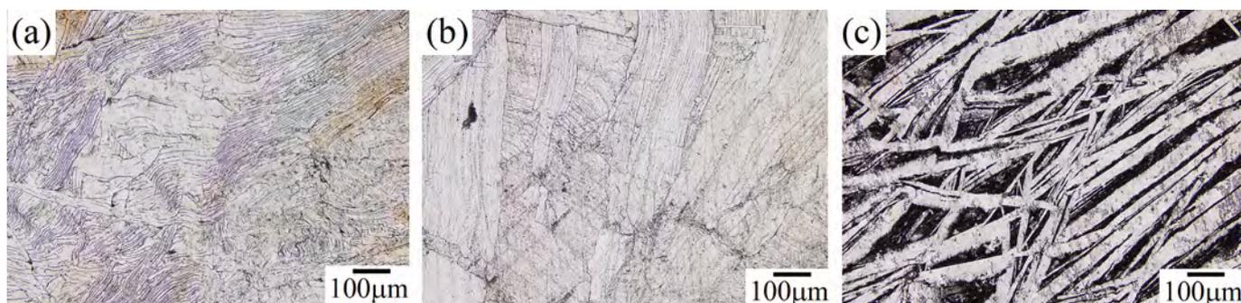
Fig. 3. Microstructure of the etched samples for (a) undoped  $\text{Bi}_2\text{Te}_3$  (b)  $\text{Bi}_{0.4}\text{Sb}_{1.6}\text{Te}_3$  and (c)  $\text{Bi}_2\text{Te}_{2.55}\text{Se}_{0.45}$ .
