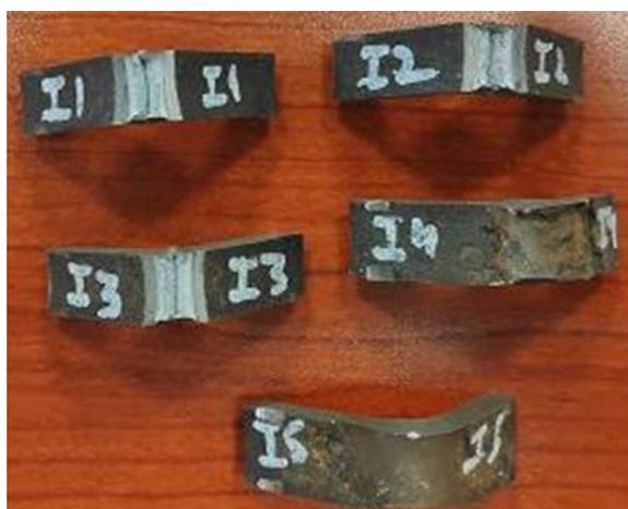
**Figure 10.** Charpy specimens after the test.
